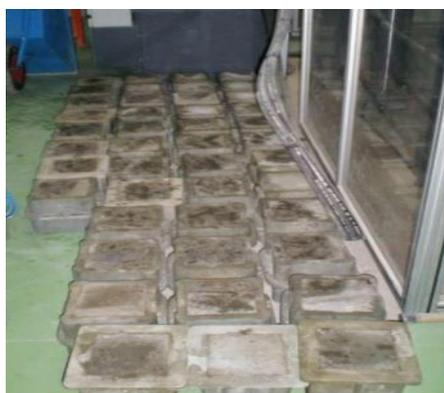
Figure 3. Casting cubes of different concrete mixtures
