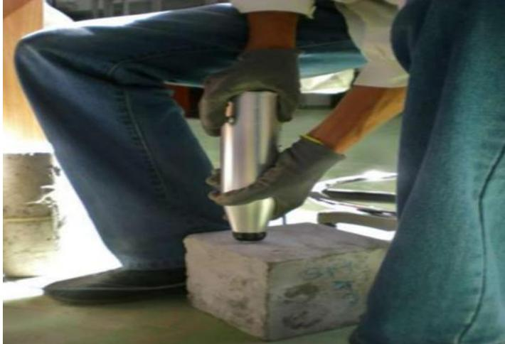
Figure 7. Schmidt's hammer measurement on concrete specimen
