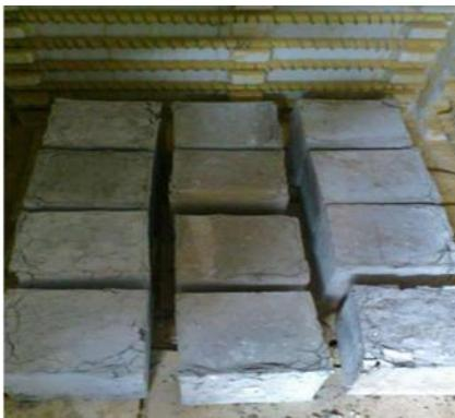
Figure 5. Process of cooling concrete samples
