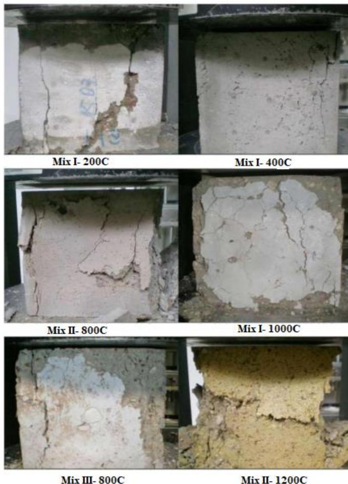
Figure 10. Images of failure under the influence of axial compression of the tested samples
