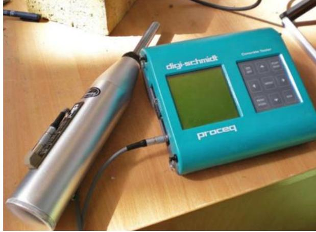
Figure 6.Schmidt's hammer for Sclerometric examinations
