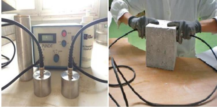
Figure 8. Test setting and measurements of ultrasonic waves
